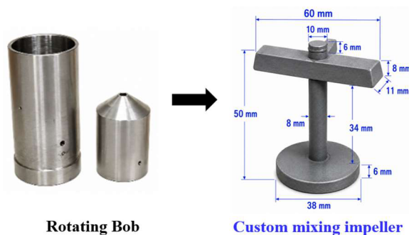
Figure 3. Custom mixing impeller used for continuous laboratory-scale shearing of mayonnaise in the modified viscometer. The principal geometric dimensions are indicated in the figure.
